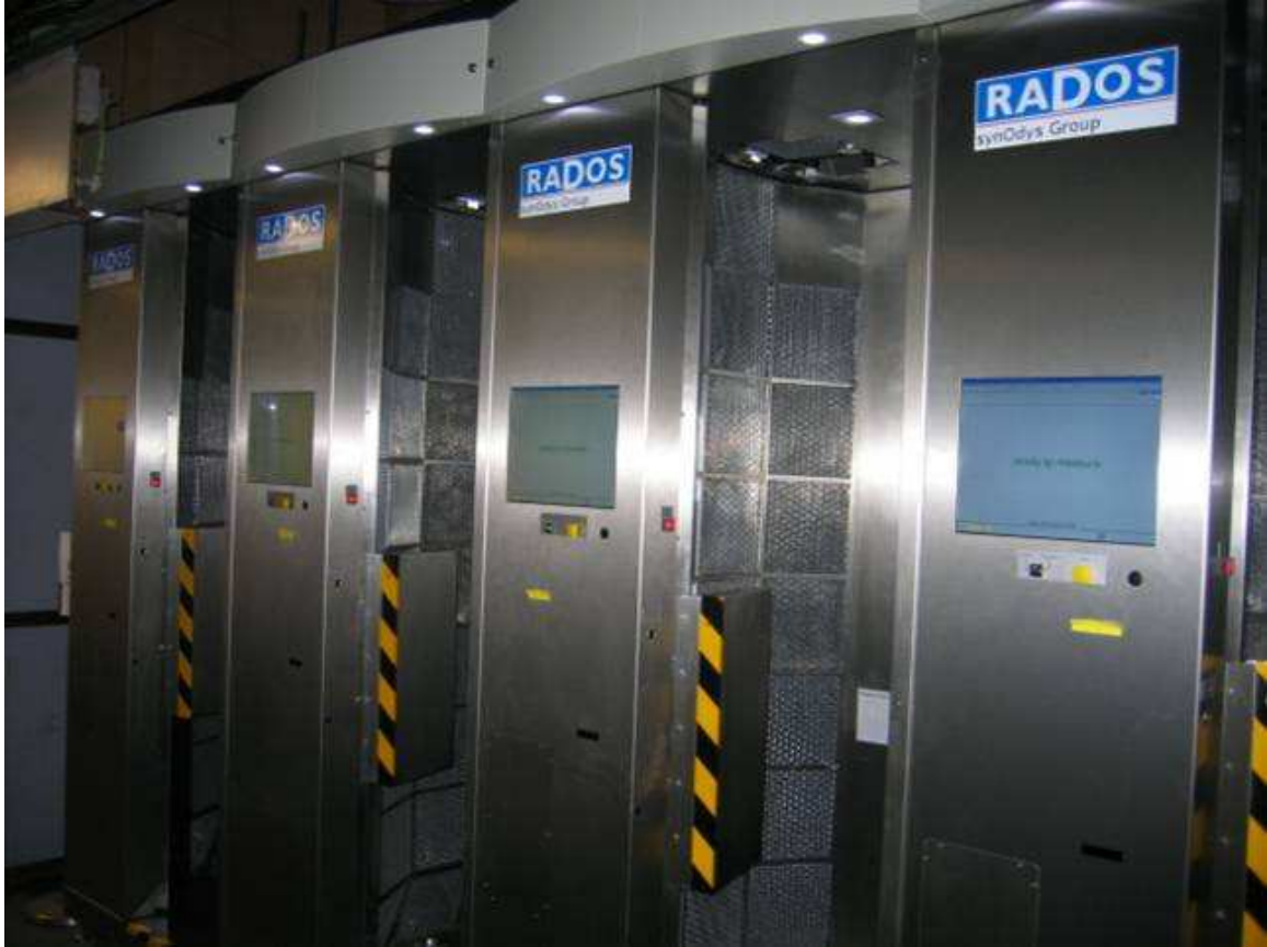
The Two-Step Exit monitors installed at Wylfa Power Station
